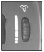
The thumbwheel for this feature is located on the instrument panel to the left of the steering column.
